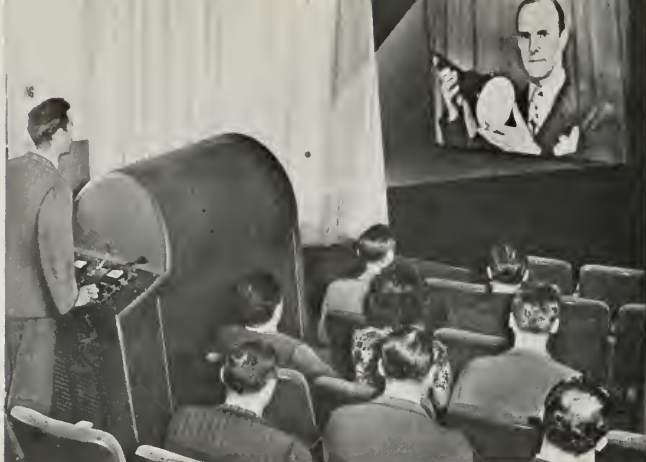
DEMONSTRATION OF LARGE SCREEN TELEVISION PROJECTION, PROVIDING A SCREEN PICTURE 6 BY 8 FEET.
