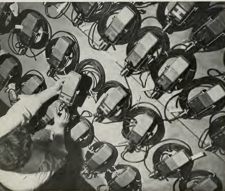
MICROPHONES USING THE PERMANENT MAGNET PRINCIPLE OF OPERATION UNDERGO FINAL INSPECTION AT THE RCA PLANT IN CAMDEN.
